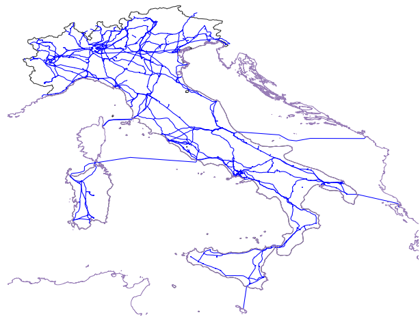
Figure 1 Italian high-voltage ( \geq 220\text{kV} ) transmission network.
